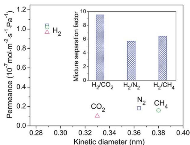
**Fig. 9** Permeances of binary gas mixtures (triangles:  $\text{H}_2\text{-CO}_2$ , squares:  $\text{H}_2\text{-N}_2$ , circles:  $\text{H}_2\text{-CH}_4$  with an equal volume ratio) through the ZIF-78 membranes at 25 °C as a function of molecular kinetic diameters. The inset shows the mixture separation factors for  $\text{H}_2$  over  $\text{CO}_2$ ,  $\text{N}_2$  and  $\text{CH}_4$ .
