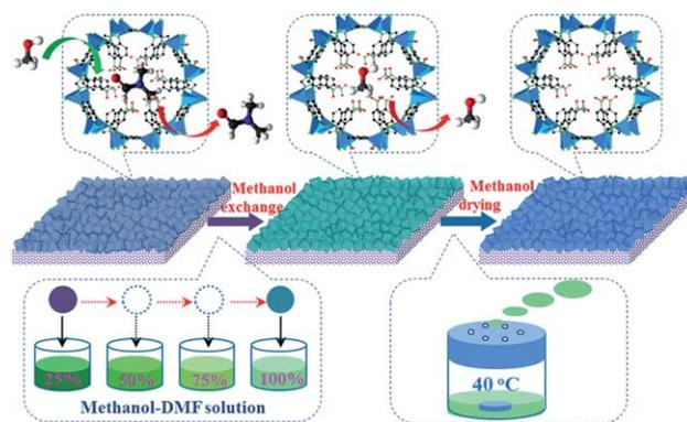
Fig. 1 Schematic diagram of the activating process of the ZIF-78 membrane.
