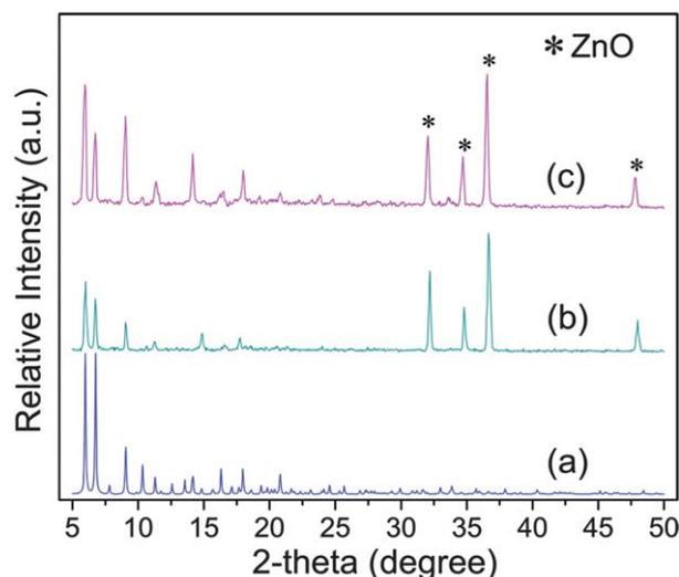
Fig. 2 XRD patterns of (a) the simulated diffraction data of ZIF-78; (b) ZIF-78 seed layer on a zinc oxide support; and (c) the as-prepared ZIF-78 membrane.
