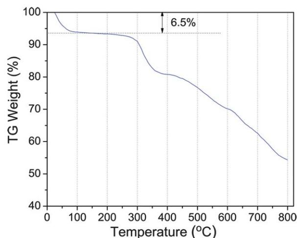
**Fig. 6** TG curve of the as-prepared ZIF-78 powder.
