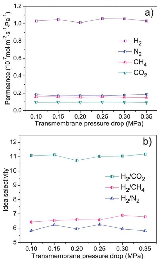
**Fig. 8** (a) Single gas permeances of  $\text{H}_2$ ,  $\text{N}_2$ ,  $\text{CH}_4$  and  $\text{CO}_2$  through the ZIF-78 membrane as a function of trans-membrane pressure drops at 25 °C; (b) the ideal selectivities of  $\text{H}_2\text{-CO}_2$ ,  $\text{H}_2\text{-CH}_4$ , and  $\text{H}_2\text{-N}_2$  for the ZIF-78 membrane as a function of trans-membrane pressure drops at 25 °C.
