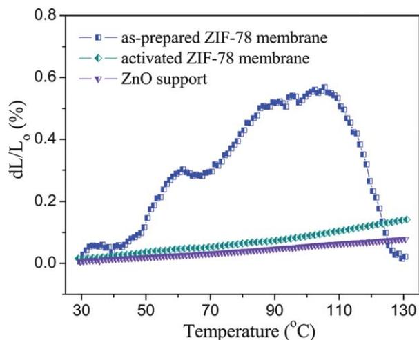
**Fig. 5** Expansion behavior of the ZnO support, and the as-prepared and activated ZIF-78 membranes in an air atmosphere.
