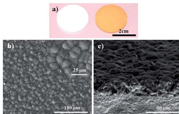
**Fig. 7** (a) Digital photos of the ZnO support (left) and the activated ZIF-78 membrane (right); SEM images of the activated ZIF-78 membrane surface (b) and cross-section (c).
