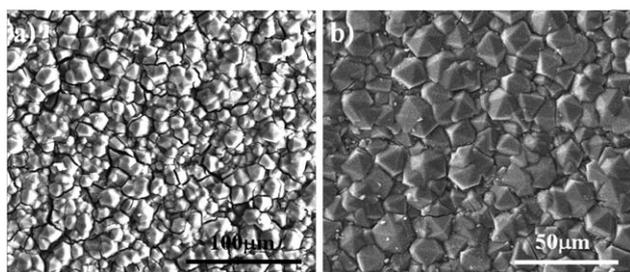
**Fig. 4** SEM images of the ZIF-78 membranes activated (a) at 100 °C and under vacuum for 12 h; (b) by methanol exchange for 12 h, and then dried at 60 °C under vacuum.
