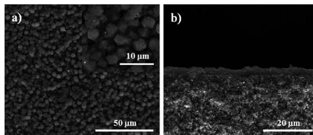
Fig. 3 SEM images of the ZIF-78 seed layer: surface (a) and cross-section (b).
